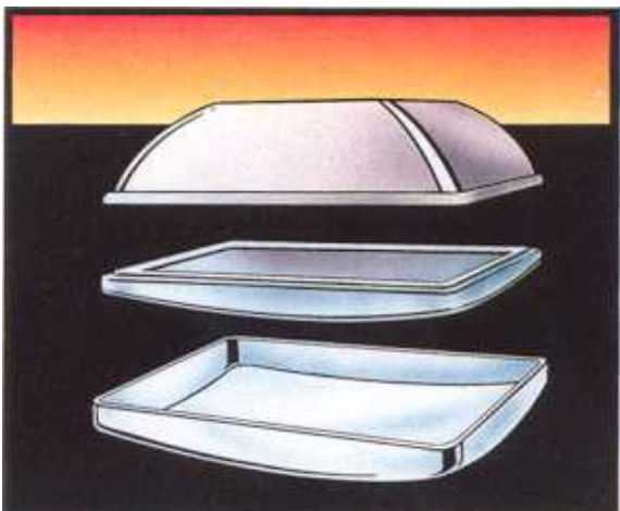
9 Assembly of screen, mask, and inner cone
