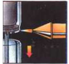
13 Sealing-in of the electron gun
