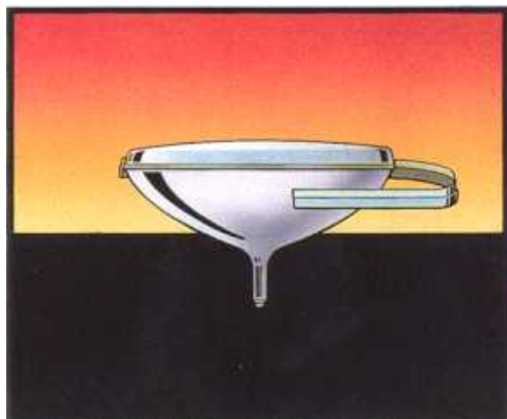
15 Application of the rimband
