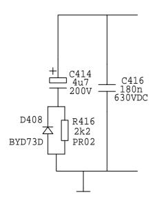
An additional damper for the horizontal deflection cannot be combined with the largest S-correction capacitor. Therefor an additional damper is necessary as drawn in the circuit diagram on the left hand side.
