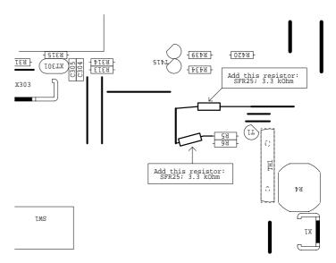
The outputs P0.5 pin 16 and P0.7 pin 14 of IC304 respectively signal "DEGS" and "DPMS" should be equipped with a pull-up resistor of 3k3 to +5 Volt. These resistors are not present in the lay-out. Best location to add these resistors is near R5 and R6 according to the drawing on the right:
