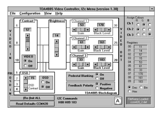
I<sup>2</sup>C-CONTROL MENU OF THE D-A CONVERTER IC TDA8447
