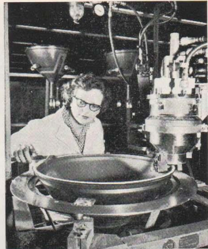
Fig. 8. The phosphor panel and shadow mask are joined to tube funnel with a soft glass called frit. Heating the junction makes permanent, strong seal.
